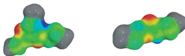
Figure 14. Left: Biuret group (based on HDI; HDI = 1,6-hexamethylene diisocyanate) \mu = 3.3 . Right: Urethane (based on HDI) \mu = 2.4 Debye. [18]
